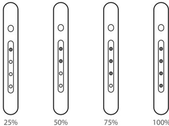
There are 4 power indicator lights located on the power bank. Each represent the battery level.
