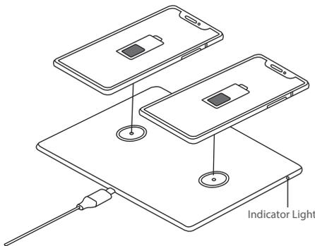
There are two charging coils on the wireless charging base. Their positions are marked on the surface, you can place your devices accordingly. The base can fast charge two devices at the same time. The indicator light showcases when the device is properly being charged.
