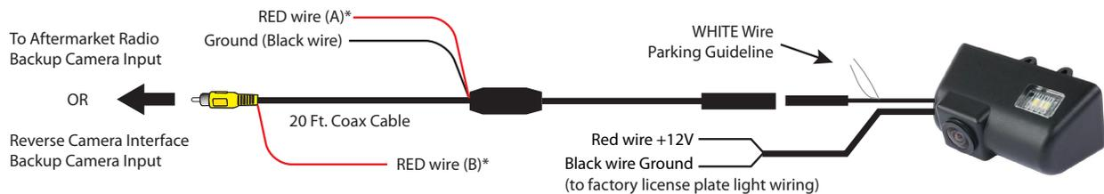
**\*NOTE:** To power the camera, use RED Wire A or B. If tapping power from the radio or RVC Interface, make sure to insulate RED Wire A to avoid it from shorting. If you will be tapping power from the reverse light +12V, insulate RED Wire B to avoid it from shorting. With either connection the Black GROUND wire needs to be connected to a solid chassis ground. For vehicles with manual transmission, we recommend tapping +12V power from the reverse light.
