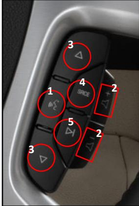
\* You can enable the factory steering wheel Voice button to activate Voice Recognition (VR) on the aftermarket radio. If your radio doesn't support VR you can assign the Voice button to activate OnStar by turning on DIP switch #1 on the 3 position DIP Switch. See diagram on page 2.
