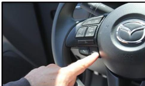
5. Press the "hang-up" button for 5 seconds to toggle to the desired AV input. Play the device.
