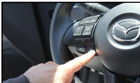
1. Press the phone "hang-up" button for 5 seconds to toggle between Navigation and video inputs. Each toggle of the input requires the "hang-up" button to be pressed for 5 seconds.
