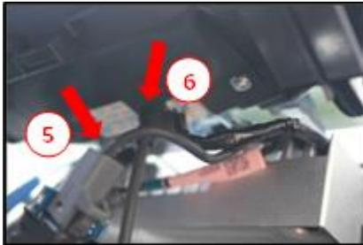
5. Unplug the factory 4-pin LVDS connector and plug it into the MZ-72A LVDS cable.
