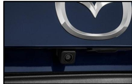
8. Install camera (sold separately) and run the camera cable to the MZ-72A module and plug to the camera input RCA.
