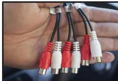
4. Plug the Audio devices to the RCA audio inputs.
