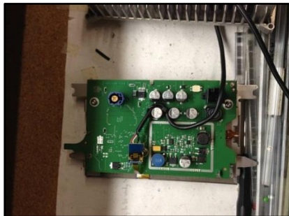
4. Plug the overlay touch screen panel ribbon cable to the connector and secure with zip tie.
