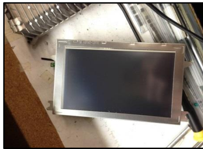
2. Remove the screen from the heat sink.
