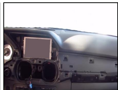
6. Connect the LVDS cable from the NAVMB-78B to the screen.
