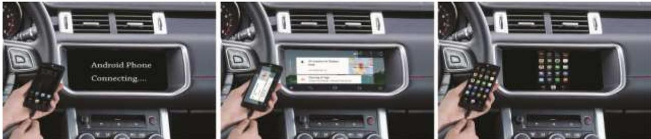
6. Connect the original USB cable to the interface’s USB extension cable and to the phone. Android Auto will be launched automatically. User may use the OE touch screen to control all the functions.
