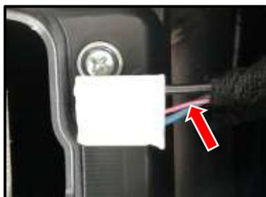
7. Tap the YELLOW ACC wire from the ACPMZ-72Z power harness to the PINK wire found on the 4 pin connector behind the radio. Be sure to tape it securely.
