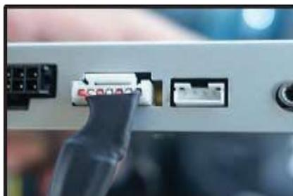
11. Plug the 6-Pin Audio Harness to the main interface module. This allows 2 audio inputs and 1 audio output.
