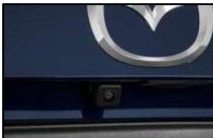
11. Install camera (sold separately) and run the camera cable to the MZ-72Z module and plug to the camera input RCA.
