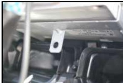
2. Remove 10mm screw to remove the radio.
