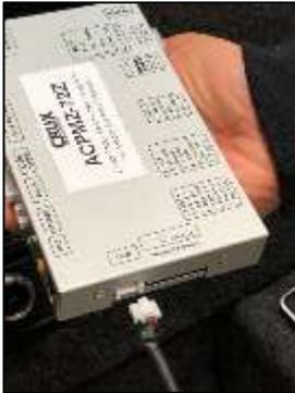
13. Plug the USB extension cable to the module and run the cable towards an easily accessible location.
