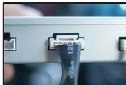
8. Plug the 6-Pin Video Harness to the main interface module. This allows 2 video and 1 reverse camera inputs.
