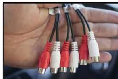
12. Plug in the audio devices to the RCA audio inputs.
