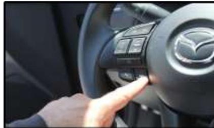
17. Press the phone "hang-up" button for 2 seconds to toggle between Android Auto and the video inputs. Each input requires the "hang-up" button to be pressed for 2 seconds.
