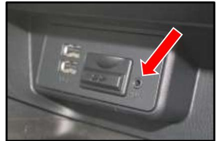
15. Plug the provided 3.5mm cable to the audio output (labeled Stereo) on the module and to the factory audio input jack of the vehicle.
