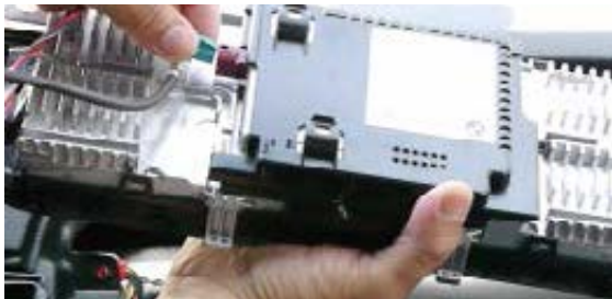
3. Plug in the Blue 6-Pin LVDS Harness from the NAVBM-77N module to the factory display unit.
