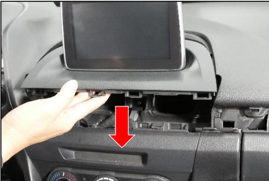
5. Once the 10mm bolt is removed, the radio screen assembly is secured with clips. Gently pull the assembly until it pops out.
