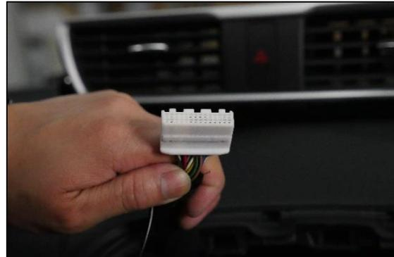
6. Unplug the 28 pin connector from behind the radio screen.
