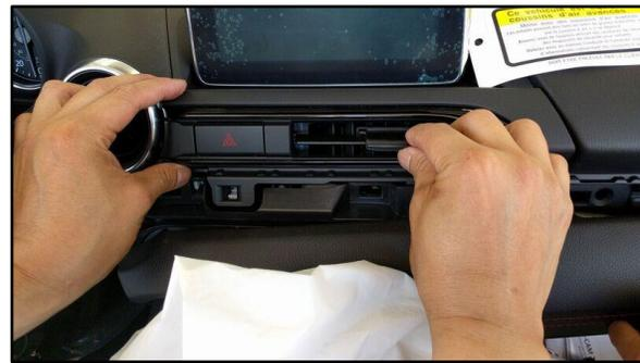
1. Partially remove dash trim below the AC vent by gently pulling towards you with a panel remover. Avoid removing it completely as it will be difficult to put back in.
