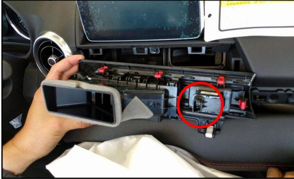
3. Unplug the hazard light connector from behind the AC vent.
