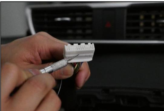
7. Release the terminal lock by pulling it up with a pry tool or any pointed tool. The terminal lock does not fully remove!
