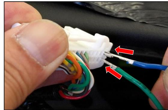
8. Connect the video output wires by inserting the BLUE wire (Video signal +) into PIN 1 and the GREEN wire (Video signal ground) into PIN 15. Make sure that the pins are inserted far enough into the connector to lock in place. Press down the terminal lock to lock pins in place.
