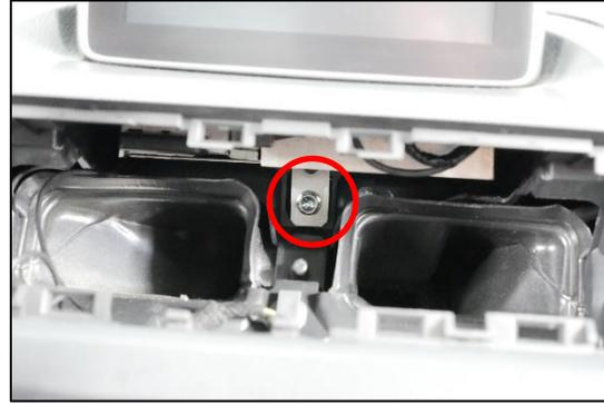
4. With the AC vent removed, unscrew the 10mm bolt holding the radio screen.
