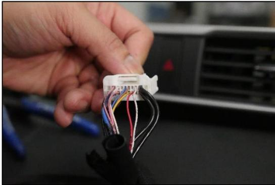
9. Unplug the 18 pin connector and locate the following wires:
