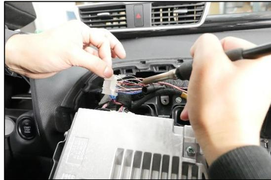
10. Tap the wires from the RVCMZ-72D module harness to the OEM connector wires according to the diagram below. We recommend soldering for a secure connection.
