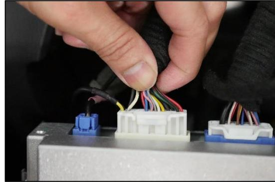
12. Plug the factory connectors back into the radio and temporarily place radio back into the dash for testing.
