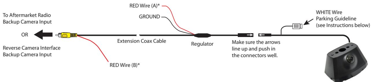
**\*NOTE:** To power the camera, use RED Wire A or B. If tapping power from the radio or RVC Interface, make sure to insulate RED Wire A to avoid it from shorting. If you will be tapping power from the reverse light +12V, insulate RED Wire B to avoid it from shorting. With either connection the Black GROUND wire needs to be connected to a solid chassis ground. For vehicles with manual transmission, we recommend tapping +12V power from the reverse light.
