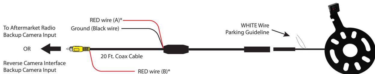
**\*NOTE:** To power the camera, use RED Wire A or B. If tapping power from the radio or RVC Interface, make sure to insulate RED Wire A to avoid it from shorting. If you will be tapping power from the reverse light +12V, insulate RED Wire B to avoid it from shorting. With either connection the Black GROUND wire needs to be connected to a solid chassis ground. For vehicles with manual transmission, we recommend tapping +12V power from the reverse light.
