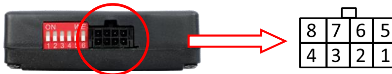
Pin assignment male 8-pin connector of VIMHK-97
